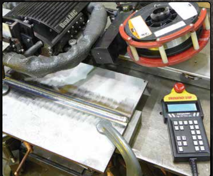
DualARC weld head mounted on flat track for weld program development tests.
