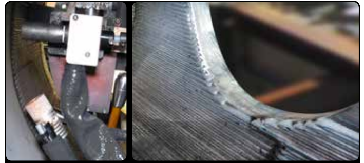
AdaptARC equipment with a custom fixture being used for a cladding operation.
