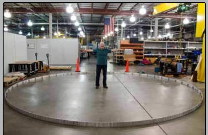
Our excellent manufacturing support produced this custom built 24' mounting track, used to construct an orbitally welded acid tank for a world class chemical producer.
