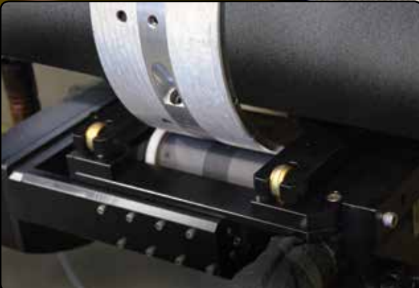
Maximum grip roller and track for secure straight or curved track operation.
